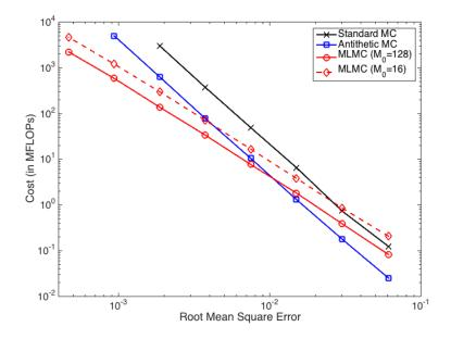
As predicted, the cost for standard and antithetic MC grows like  $TOL^{-3}$  and the cost for MLMC grows like  $TOL^{-2}$ . The actual cost depends on the choice of coarsest grid.
